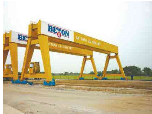
Cổng trục / Gantry Crane Quatity: 34 units Capacity: 3 - 50 tons
