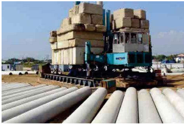
Dàn ép cọc / Pressing Rig Quatity: 06 sets Capacity: 120 - 900 tons
