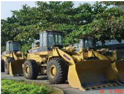
Xe xúc lật / Wheel Loader Quantity: 09 units Capacity: 2.5 - 3 m 3
